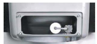
Integrated water buffer tank with float valve to prevent against any irregularities in the water supply. This reduces the risk of cavitation occurring in the pump - which is a major cause of high pressure pump failure.
